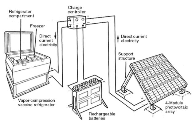
Vaccine Refrigerator Powered by a Photovoltaic System
